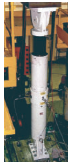
Damper test TRANSPEC® SHA
